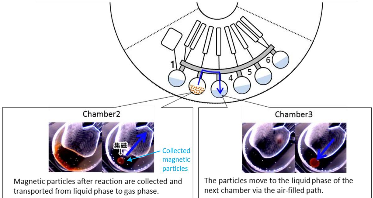
MINT technology: Schematic illustration of the transportation of magnetic particles in the cartridge
